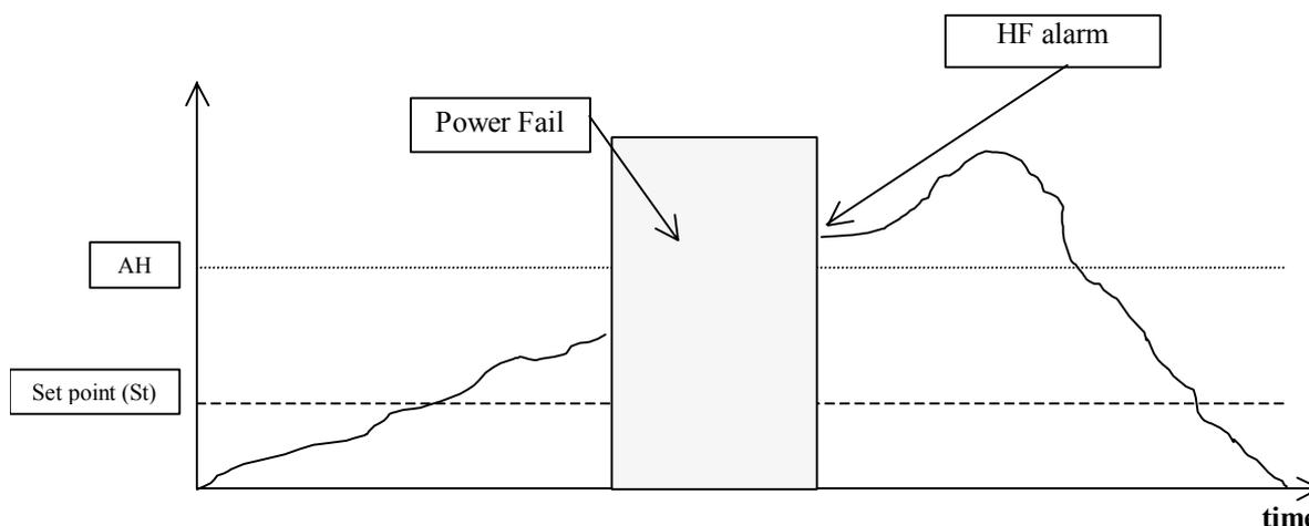
The activation of one or both of the alarms causes the  $\text{HACCP}$  LED to flash and the display of the alarm code, as well as the recording of the alarm to the  $\text{E}^2\text{PROM}$  and the activation of the alarm relay or buzzer (if present).
