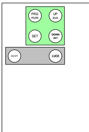
The highlighted part is used to simulate the instrument keypad from the remote control. In **Level 0** (display the reading and message 'rCt'), the following functions are active:
