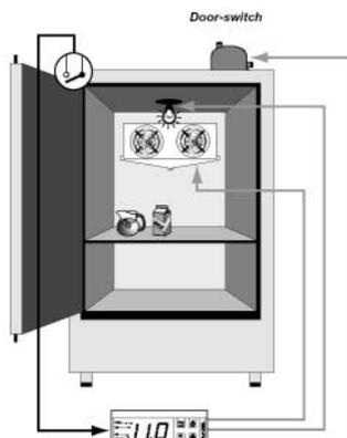
**Note:** If the light was previously switched on manually, when the door is closed the second time, it is automatically switched off.
