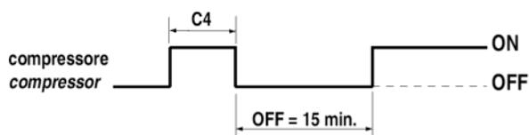
**Default:** ‘c4’=0 => compressor always Off in the event of a virtual control probe error.
