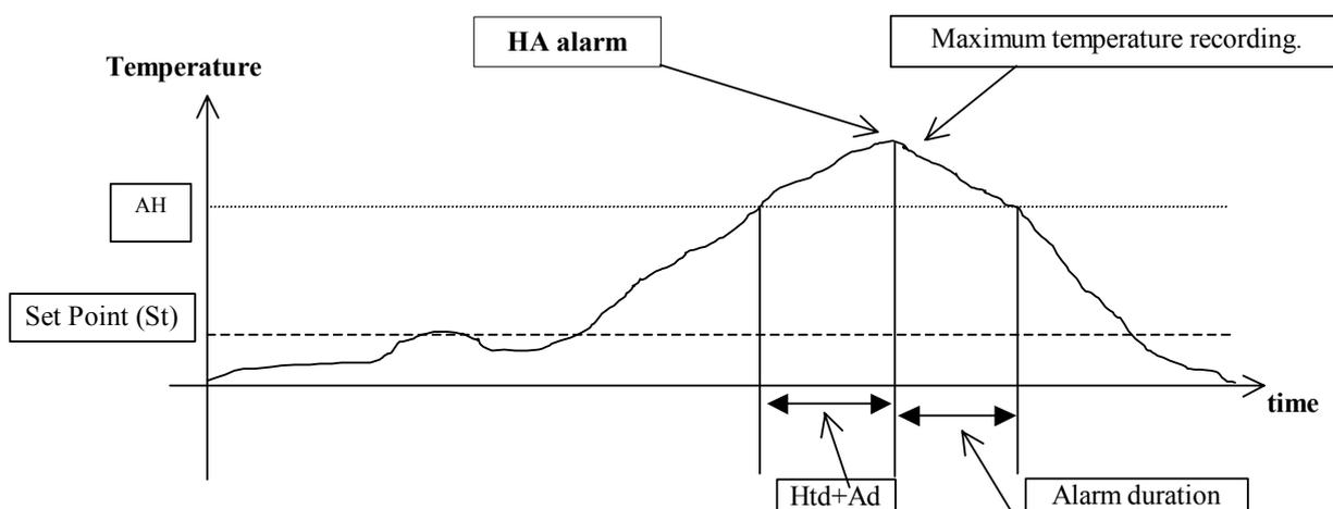
**“HF”** – this occurs after a power failure for an extended time ( $>1$  minute) if, when power returns, the temperature is higher than the threshold set for the parameter “AH”: the absolute value of AH, if “A1”= 0; the relative value given by “AH” + “St”, if “A1”= 1.
