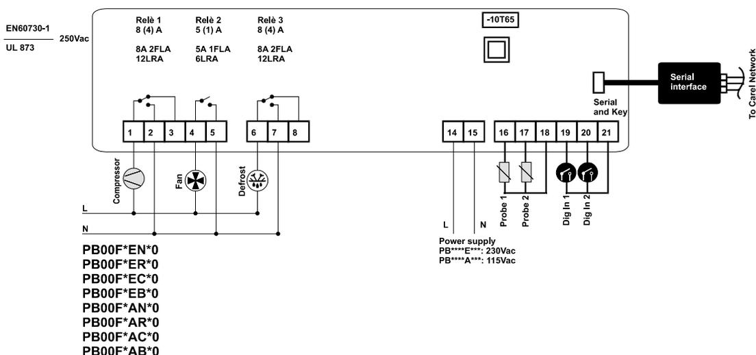
powercompact connections: 230 Vac or 115 Vac with transformer and 16 A relay version
