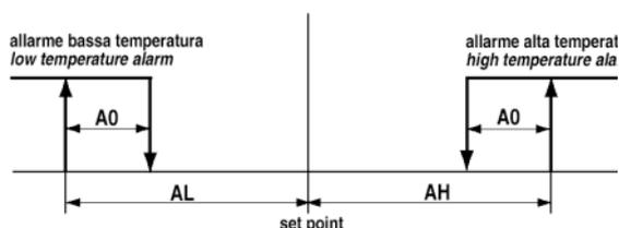
This represents the differential used in the activation of the high and low temperature alarms ('AL' and 'AH') (see the figure shown below) and for the management of the fans (see the F parameters). In the event of an alarm, as can be seen from the figure, the value of 'A0' affects to the determination of the effective activation points of the temperature alarm.
