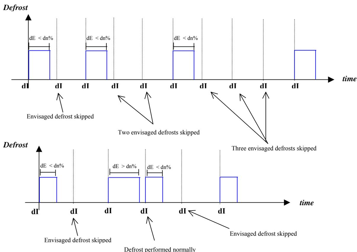
This function should be used with the progributed over the day (e.g. cyclical defrosts, parameter ‘dI’). This prevents skipping defrosts that would be the last before a long period programmed without defrosts (for example, when the clock is used to program the defrosting of the utility at night only).
