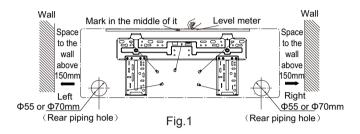
(2) Open a piping hole with the diameter of  $\Phi$ 55mm(70mm) on the selected outlet pipe position.In order to drain smoothly, slant the piping hole on the wall slightly downward to the outdoor side with the gradient of 5-10°.(As show in Fig.2)
