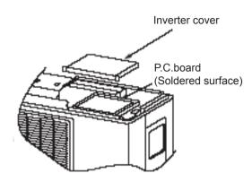
(2)As shown below, connect the discharge resistance (approx.  $100\Omega20W$ ) or plug of the sold ering iron to voltage between + - terminals of the electrolytic capacitor on PC Board for 30s, and then performed is charging.
