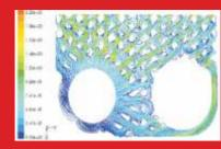
Simulation is one of the most important stages in the development of new and existing BPHEs. The ability to evaluate different plate patterns by simulating flow international bodies, such as PED, UL, KHK rate and directions offers great opportunities for improved functionality.
