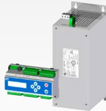
The GMM phase cut is used for voltage-controllable AC external rotor motors. This is the most cost-effective way of realising a speed controller, while achieving constant pressure conditions in the cooling circuit. Utilization is not recommended for noise-sensitive applications or applications with stringent energy efficiency requirements. High operational reliability can be achieved with this product's integrated bypass function.
