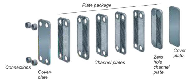
The fluids can pass through the heat exchanger in different ways. For parallel flow BPHEs, there are two different flow configurations: cocurrent or counter-current.
