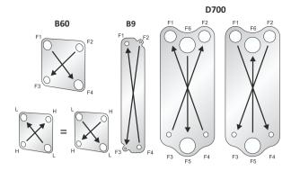
The B9, B60 and D700 have a cross-flow configuration, instead of the parallel flow normally found in BPHEs. In the B9 and B60, ports F1-F4 are equivalent to the outer circuit, and ports F2-F3 to the inner circuit. For the D700, ports F5-F6 are the outer circuit and ports F1-F4 and F2-F3 are the inner circuits.
